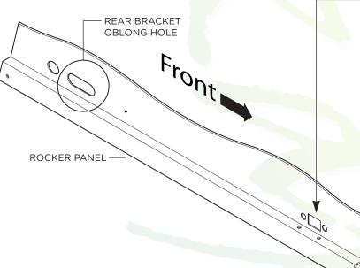
**6.**Locate the rectangular slots and holes on the Rocker Panel. Install the U-Nut Clips as shown (6a, 6b). Make sure that the threads of the U-Nut Clips are to the inside of the Rocker Panel. Be careful not to drop the U-Nut Clips inside of the Rocker Panel.
