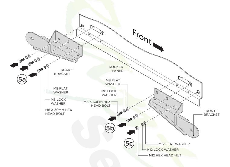
**6.** Fasten the bottom of the Front and Rear Brackets onto the Rocker Panel and fasten using two (2) M8 Hex Head Bolts, four (4) M8 Lock Washers and four (4) M8 Flat Washers and two (2) M8 Hex Head Nuts per bracket.
