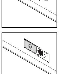
**4.** Locate the hole near the front of Rocker Panel. Place the Bolt Plate through the hole in the Rocker Panel as shown (4a thru 4c).
