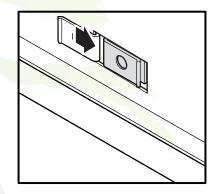
**5.** Place the Rear Bracket onto the Rocker Panel and fasten using two (2) M8 X 30 Hex Head Bolts, two (2) M8 Lock Washers and two (2) M8 Flat Washers as shown (5a).
