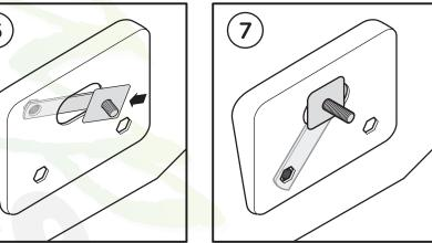
**9.** Align the Passenger Side Front Bracket with the threaded studs of the Bolt Plates and the Hex hole in the Rocker Panel. Align the Passenger Side Rear Bracket with the threaded stud of the M12 Bolt + M10 Nut Plate and fasten as shown (9b). If lower holes are pre-threaded, fasten using one (1) M8 Hex Head Bolt, one (1) M8 FLat Washer and one (1) M8 Lock Washer (9c).
