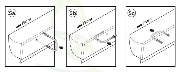
**6.** Position the Top Flange of the bracket onto the U-Bolt. Secure the Mounting Bracket to the U-Bolt using two (2) M8 Flat Washers, two (2) M8 Lock Washers and two (2) M8 Hex Head Nuts as shown and leave loose.
