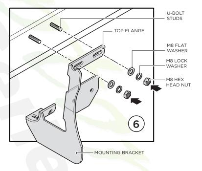
**7.** Secure the Backing Plate to the Mounting Bracket using two (2) M8 X 30MM Hex Head Bolts, four (4) M8 Flat Washers, two (2) M8 Lock Washers and two (2) M8 Hex Head Nuts as shown and leave loose. The Backing Plate will clamp the Mounting Bracket and pinch weld together. Repeat steps 4 through 7 for Rear Bracket.
