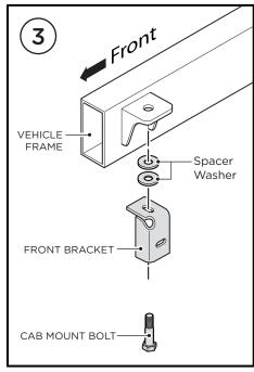
Note: Make sure existing washer and rubber bushing is in place.
