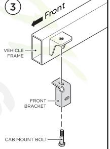
**Note:** Make sure existing washer and rubber bushing is in place.
