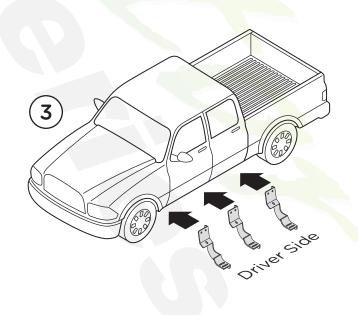
4. Align the Front, Center and Rear Driver's Side Brackets with
