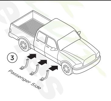
**4.** All passenger side Brackets are identical with the bracket cradle facing toward the rear of the vehicle. Install the first passenger side Bracket should be first passeng the first passenger side Bracket closest to the front wheel. Align with existing factory holes in the rocker panel as shown (4a), Secure the first Bracket using one (1) M8 x 30mm Hex Bolt, one (1) M8 Lock Washer and one (1) M8 Flat Washer (4b).
