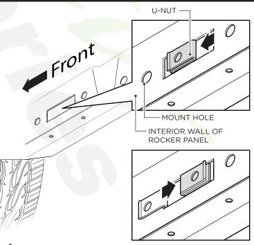
**3.** On the passenger side of the vehicle, align the Front and Rear Brackets as shown.
