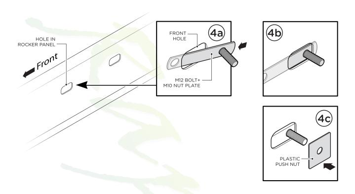
**5.** Locate hole in the rocker panel and insert one (1) Bolt Plate with M12 Stud into the hole (5a) and (5b). Slide Plastic Push Nut over the Stud (5c). Repeat for Rear Bracket.
