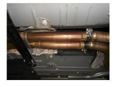
2) Begin by placing a supplied 2 ½" clamp onto each of the slip fits on Scavenger pipe #86331S. Place the Scavenger pipe onto the back of the stock head pipes (make sure the Flowmaster embossing is facing the ground). Level and center the assembly in the drive line tunnel and support with a stand. Tighten the two clamps enough to hold, but still allow for adjustment. Reinstall the two body braces onto the vehicle and tighten securely.
