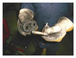
3) To install the new Flowmaster system you will need to remove the factory hanger located on the cross member just behind the rear differential. After unbolting the hanger, remove the rubber isolator from the hanger mount, the rubber isolator and the bolt securing the hanger will be re-used with the Flowmaster system.
