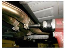
3) Support the rear of the system with a stand. Starting at the rear of the vehicle, remove the hangers on the system from the rubber mounts on the vehicle. Unclip the ground strap from the middle hanger on the right tailpipe, using a 15mm socket loosen the clamps at the slip fit connections behind the catalytic converters. Then, with the help of an assistant, lower the stand and slide the system back off of the head pipes. Carefully lower from the vehicle.
