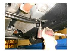
2) Using a 13mm socket, unbolt the two body braces in the center of the vehicle.
