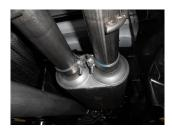
9) Install a provided  $2\frac{1}{2}$ " clamp onto the left muffler outlet. Place the front section of the left side tailpipe **#86194S** into the left side muffler outlet and connect the hanger on the pipe to the rubber mount on the vehicle. Tighten the clamp enough to hold, but still allow for adjustment. Place a second  $2\frac{1}{2}$ " onto the back of this pipe in preparation for the next step.
