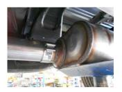
4) Place a supplied 3" clamp over the inlet of the muffler, then slide the inlet of muffler onto the back of the inlet pipe. Use a stand to support the muffler. Tighten the clamp just enough to hold in position.
