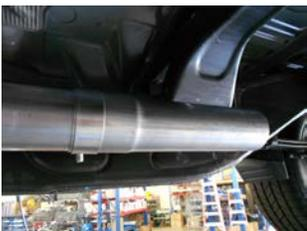
2) If installing the system on a truck with a 6.5' bed, place extension pipe **#TB700S** onto the back of the **#26409S** inlet pipe, place a provided clamp onto the slip-fit and tighten enough to hold in position.
