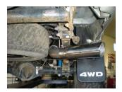
8) Place the ST429 stainless tip onto the end of the tailpipe and adjust to the desired location. Tighten the nut on the clamp to secure the tip in place.
