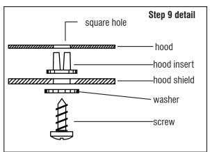
**IMPORTANT:** Before driving, ensure the hood shield is properly secured to vehicle. Clean with a **SOFT** cloth and soap and water ONLY! Using abrasive cleaners, chemicals, or solvents will **VOID** the warranty on this product.
