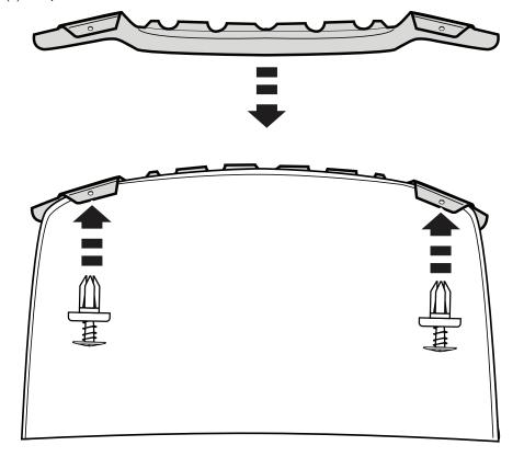
**IMPORTANT:** Before driving, ensure the hood shield is properly secured to vehicle. Clean with a **SOFT** cloth and soap and water ONLY! Using abrasive cleaners, chemicals, or solvents will **VOID** the warranty on this product.
