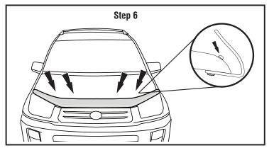
**IMPORTANT:** Before driving, ensure the hood shield is properly secured to vehicle. Clean with a **SOFT** cloth and soap and water ONLY! Using abrasive cleaners, chemicals, or solvents will **VOID** the warranty on this product.
