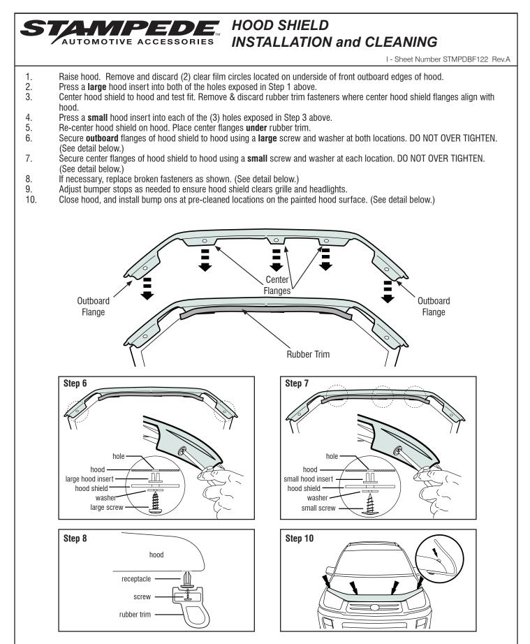
**IMPORTANT:** Before driving, ensure the hood shield is properly secured to vehicle. Clean with a **SOFT** cloth and soap and water ONLY! Using abrasive cleaners, chemicals, or solvents will **VOID** the warranty on this product.
