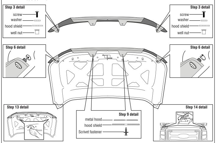
**IMPORTANT:** Before driving, ensure the hood shield is properly secured to vehicle. Clean with a **SOFT** cloth and soap and water ONLY! Using abrasive cleaners, chemicals, or solvents will **VOID** the warranty on this product.
