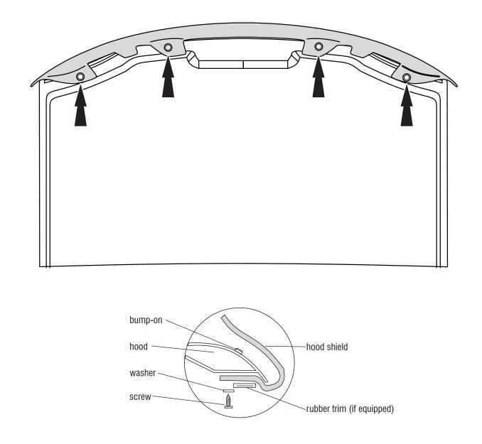
**IMPORTANT:** Before driving, ensure the hood shield is properly secured to vehicle. Clean with a **SOFT** cloth and soap and water ONLY! Using abrasive cleaners, chemicals, or solvents will **VOID** the warranty on this product.
