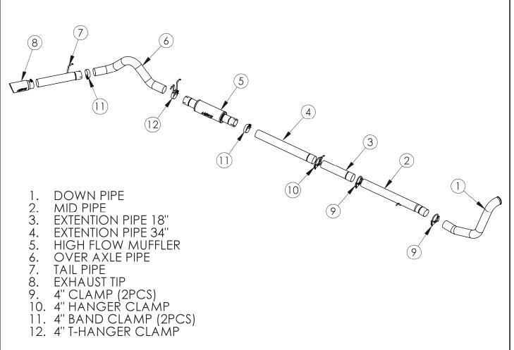
\*MUFFLER MAY NOT BE EXACTLY AS SHOWN
