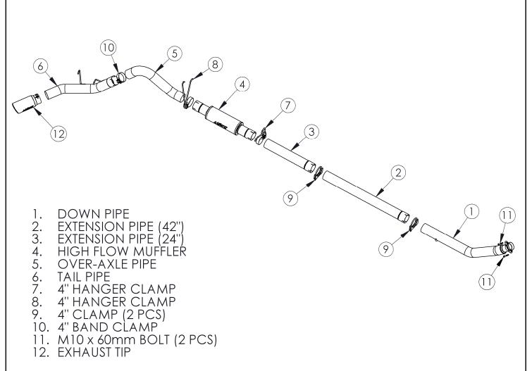
\*NOTE: MUFFLER MAY NOT BE EXACTLY AS SHOWN
