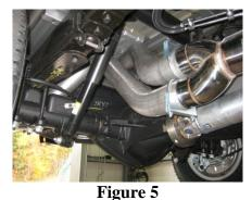
2. Use the 4" Hanger Clamp to install the Over Axle Pipe to the Y-Pipe. The expanded end slides over the upper outlet of the **Y-Pipe**. Refer to Figure 5 & 6.
