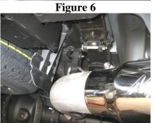
5. Install the **Hanger Kit** on the frame in the large existing hole as shown. Secure with the supplied 3/8" hardware, refer to Detail A in the Illustration. Refer to Figures 8. Note: the 3/8" x 1" Hex bolt will be used with a 3500 Dual Wheeled vehicle and be mounted through the inside frame rail only.
