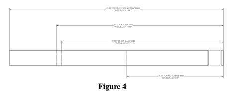
1. Install the **Extension Pipe** to the existing flange using the clamp removed earlier. Leave the hardware loose enough for some adjustment. **Refer to Figure 3**. The **Extension Pipe** will not need cutting for the Crew Cab short bed or the Extended Cab long bed. Refer to **Figure 4** for cut lengths. (**Installation tip:** Temporarily hang the **Muffler** and the **Over Axle Tail Pipe** in place and measure to the back of the Catalytic Converter to verify the length required).
