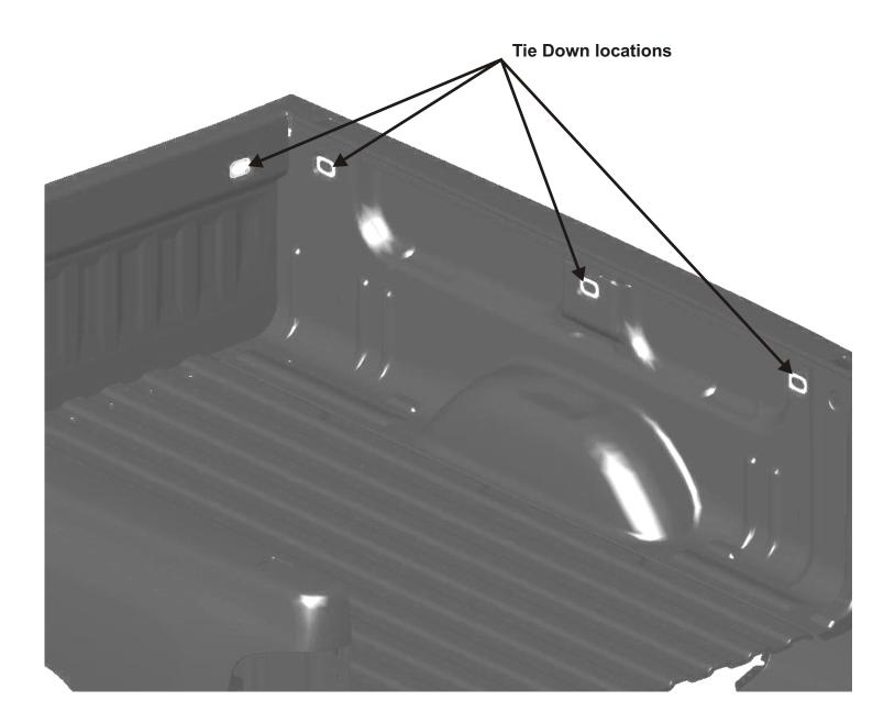
Step 2: Attach the 8mm bolt and 8mm threaded plate to the tie down as shown in the image below. With the plate towards the end of the bolt and in the rotated position as shown, insert the tie down assembly into the hole of the vehicle where the cover was removed.
