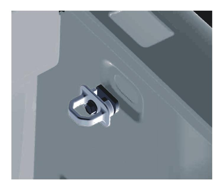
Tighten the bolt down by hand. Ensure that the plate has rotated in between the legs of the tie down to ensure a tight fit (refer to the image below). Once tight to the vehicle, torque the bolt down with a 13mm wrench to 16ft/lbs.
