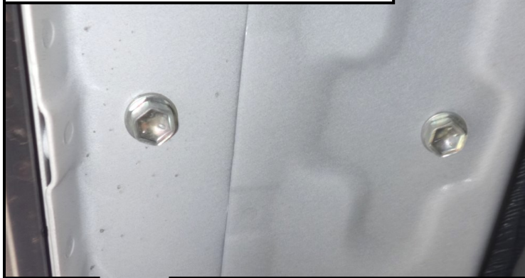
Figure 2 Driver side front rocker panel cap screws
