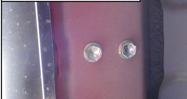
Figure 4 Driver side rear rocker panel cap screws
