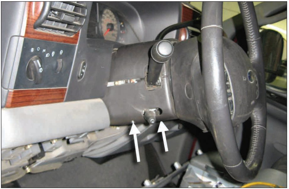
Figure 19 Remove column panel covers
