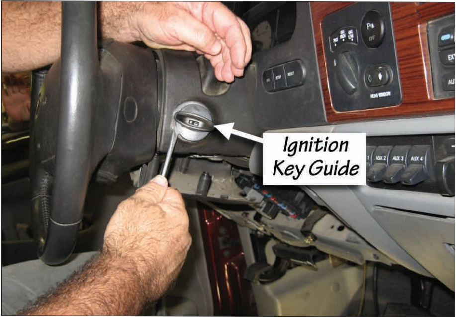
Figure 20 Remove Plastic Ignition Key Guide
