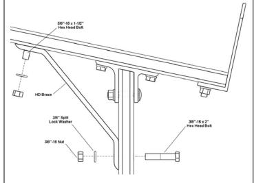
Tightening the 3/8"-16 x 2" hex head bolt first and then the nut on 3/8"-16 x 1-1/2" hex head bolt in the crossbar.
