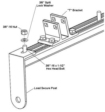
Place the adjustable load secure post onto the furthest out 3/8"-16 x 1-1/2" hex bolt in the center channel of the crossbar as shown.
