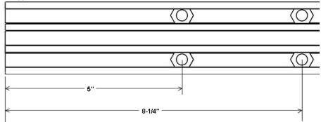
Orientate the "T" bracket as shown below; note which way the angles point. Position the "T" bracket over the nuts and install using (4) 3/8"-16 x 1" hex bolts and (4) 3/8" split lock washers. Adjust the "T" bracket so that the edge is 4.5" from the end of the crossbar. Tighten the all holts
