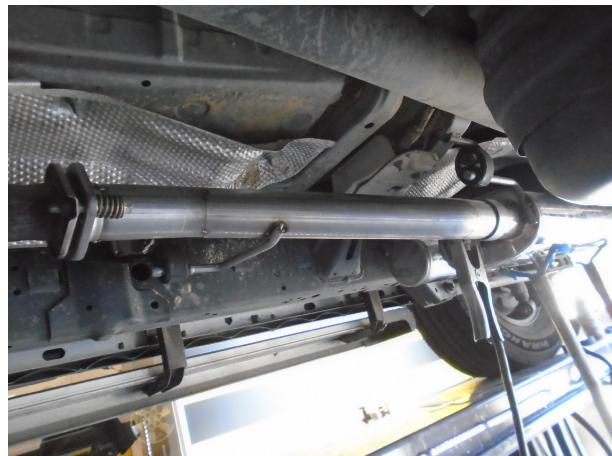
**Step 2:** Begin Installing the new system by attaching the inlet pipe to the Catalytic Converter outlet using the OE spring bolts.
