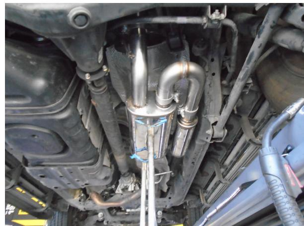
**Step 3:** Next attach the Oval Muffler to the Inlet Pipe with the supplied 2.50" clamp. This exhaust system is configured to allow the user to tune the sound. For a more moderate exhaust tone install the U-pipe Assy and the 4.00" NDT (No Drone Technology) Chamber (as shown) using the supplied 2.50" clamps. For a more aggressive sound see configuration chart below.
