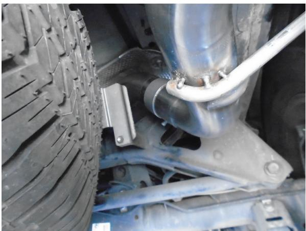
Next, loosely attach the Mid-Pipe to the muffler outlet using a supplied 2.50" clamp.
