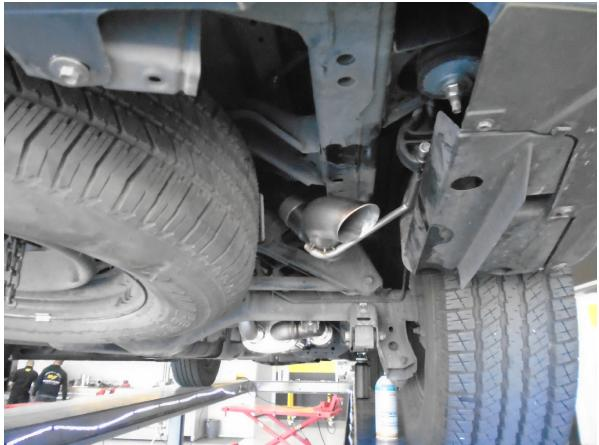
Complete the assembly by loosely attaching the Tailpipe Assembly to the Mid-Pipe using a supplied 2.50" clamp and inserting the hanger into the rubber insulator.
