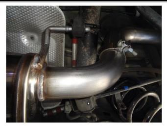
**Step 5:** Next, attach the Overaxle pipe to the muffler Assembly and loosely tighten.
