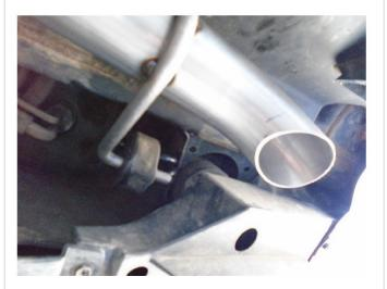
**Step 6:** Using the OE rubber insulators install the tailpipe assemblies to the Over Axle Pipe fitting the hangers into the installed hanger brackets.
