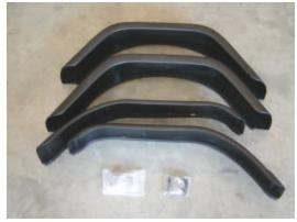
The flare kit includes: 1 each of Left and Right front flares, Left and Right rear flares, and the required hardware to install the flares.
