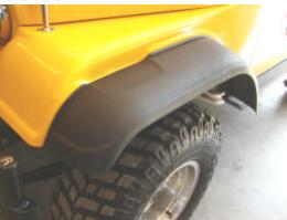
The new flare bolts in place easily and quickly utilizing the existing holes from the OE flare. This is the left front. Simply repeat the process on the right side and you're halfway finished.
