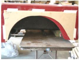
Only the rear half of the CJ wheel opening needs to be enlarged. Notice the large amount of added clearance the new flare will provide. Mark the area and cut as required.
