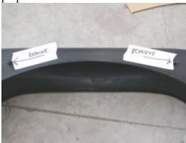
It is necessary to remove the two (2) locating studs from the rear flares. The studs are only used on TJs, and are not
