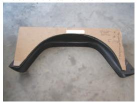
This cardboard pattern provides an outline of how the CJ rear wheel opening needs to be modified. Just be sure to properly mark the front and back and the proper orientation (left and right) before making any cuts.
