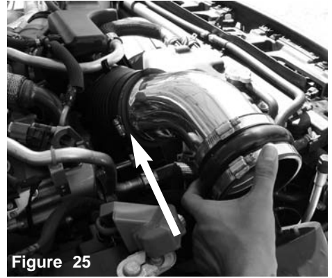
Figure 25 Install intake tube into vehicle and position into factory hose and hump hose to adaptor. Make sure the larger section of the tube is connected at factory hose.
