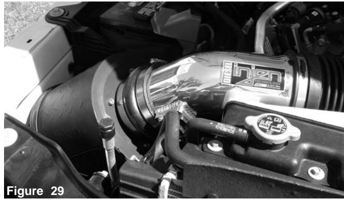
Figure 29 Check the entire system for the best possible fit. Once you have checked the entire system for leaks, rubbing or rattling, continue to tighten all nuts, bolts and clamps. Reconnect the negative battery terminal prior to starting the engine.
