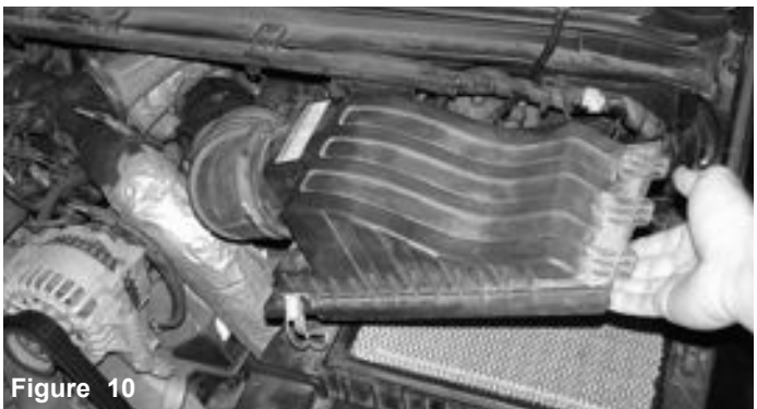
Figure 8 Unlatch the first metal clamp from the upper air box as shown above.
