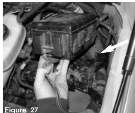
Figure 24 The small fuse box is dislodged from the stand-off located in front of the relay box.
