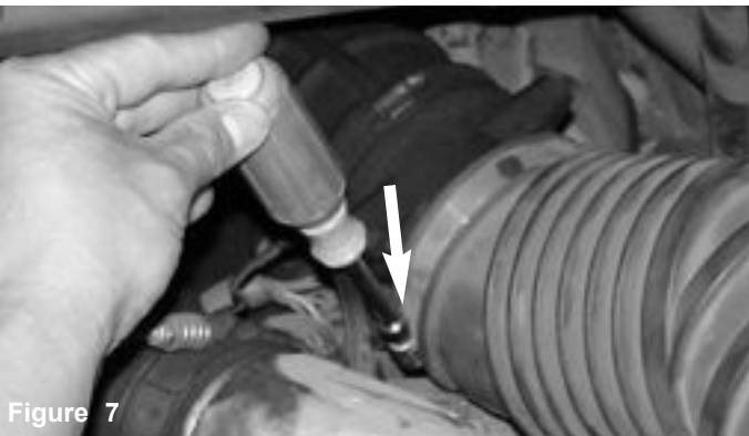
Figure 5 Pull the air restrictor gauge from the stock grommet to be used later in the instructions.
