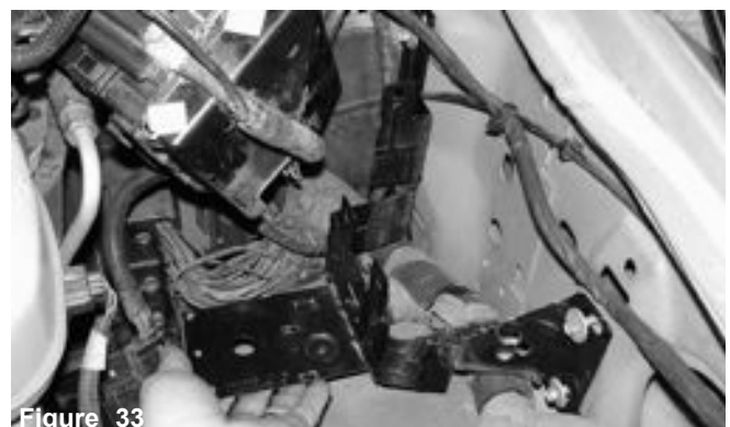
Figure 30 The stock relay bracket is ready to be pulled out of the engine compartment.
