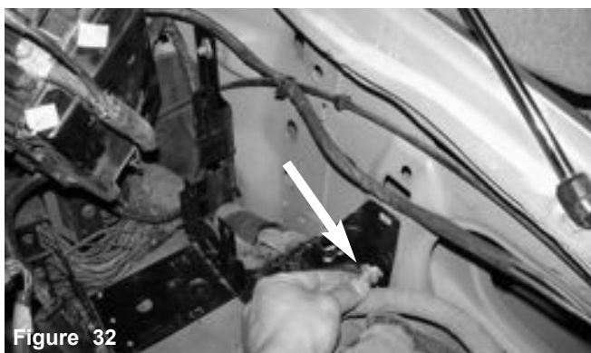
Figure 30 The stock relay bracket is ready to be pulled out of the engine compartment.
