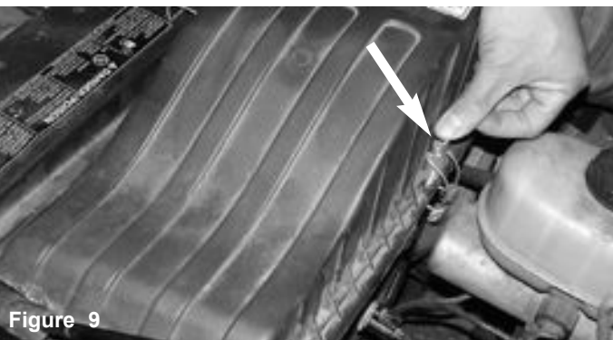
Figure 7 Loosen air duct clamp over the turbo inlet hard pipe. The air intake duct will be removed from the turbo inlet.
