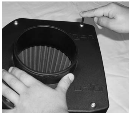
Unbolt the four- m6 x 20mm screws from the velocity stack base located to the center of the base. Now separate the base from the velocity stack.
