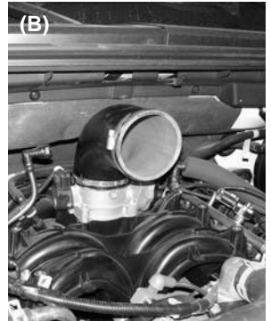
Take the 3 1/2" 90 degree elbow and two 056 clamps and insert short end of elbow over the throttle body. (Figure A) 90 degree hose shown on throttle body with both clamps loose. (Figure B)
