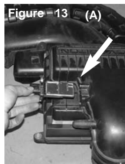
Remove the two screws that secure the MAF sensor to the stock air box and then remove the MAF sensor. (Figure A) Re-install the MAF sensor onto the machined adapter on the intake pipe. (Figure B)
