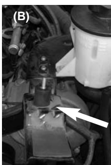
Screw the M6 vibra-mount on to the factory air box bracket (Figure A) Vibra-Mount mounted on to bracket. (Figure B)
