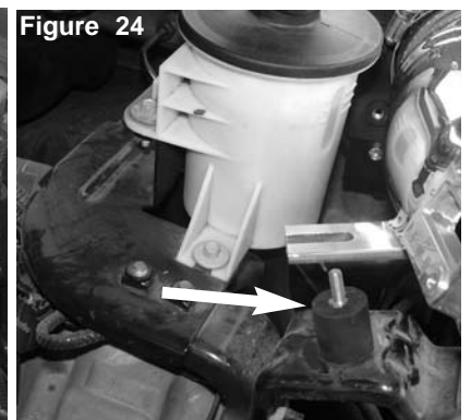
Align intake bracket to the vibra-mount stud until in seats flush to the vibra-mount.
