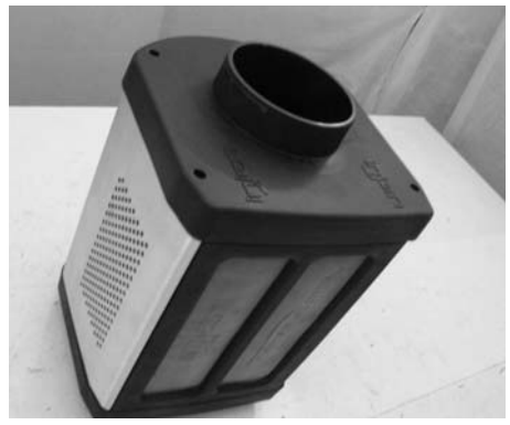
The four m6 x m20 bolts have been removed from the top of the velocity stack,
