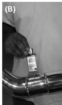
Remove the two screws that secure the MAF sensor to the stock air box and then remove the MAF sensor. (Figure A) Re-install the MAF sensor onto the machined adapter on the intake pipe. (Figure B)
