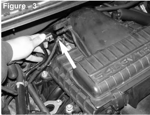
Remove the upper crank case breather line by pressing on green clip and pulling out.
