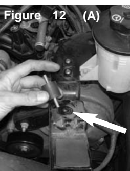
Screw the M6 vibra-mount on to the factory air box bracket (Figure A) Vibra-Mount mounted on to bracket. (Figure B)
