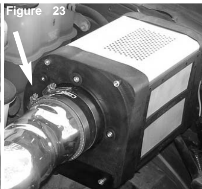
Press the 3/4" end of intake into the straight hose located on Power-box velocity stack.
