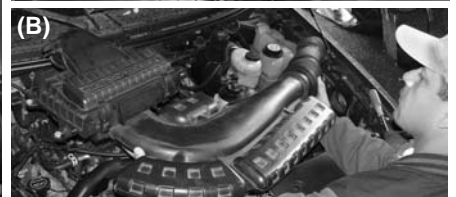
Pull the intake duct connected to the fender well to the left and pull out. (A) Remove entire air box cleaner assembly. (B)
