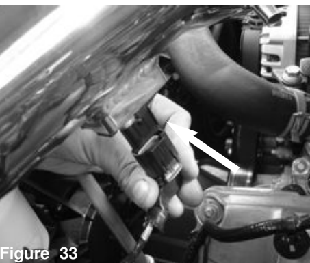
Figure 30 Slide the hump hose on to the adaptor and position.
