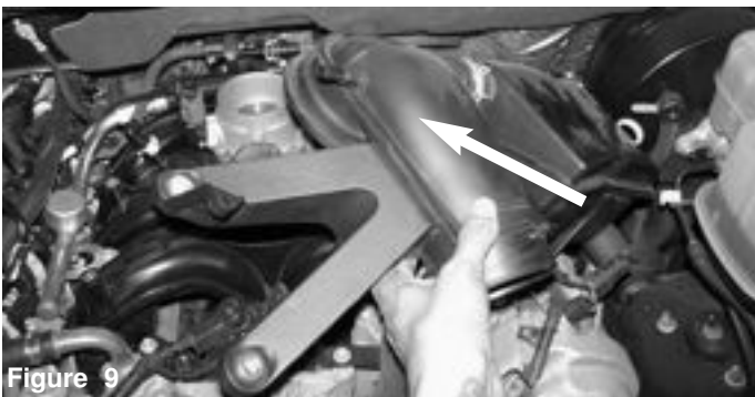
Figure 7 Loosen the four bolts holding in the resonator tube. Note: 1 bolt located under the resonator.
