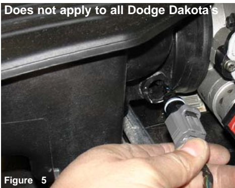
Figure 5 Does not apply to all Dodge Dakota's For those that come equipped with air temperature sensors, unplug the air temperature sensor from the intake plenum as shown above.
