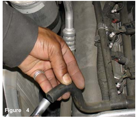
Figure 4 Disconnect the crank case vent hose from the air box cleaner port as shown above.
