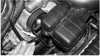
Pull the vacuum hard pipe out of the CCV box grommet as shown above.
