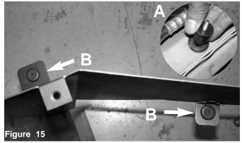
A) Install M6 thredded stand-off mount to grommet on frame. B) Attach small grommets to 1/2" hole cut-outs on heat shield tabs.
