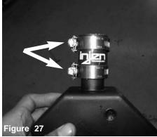
Attach the mini clamps to hose on catch can.
