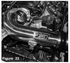
Install injen intake tube into vehicle and position to throttle body and adaptor.
