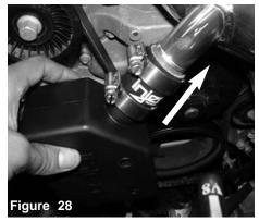
Attach catch can to fitting on intake tube.
