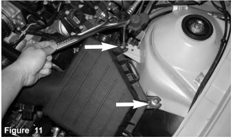
Remove the two m6 nuts holding the air box cleaner to the strut tower mount.
