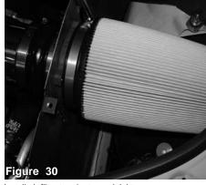
Install air filter to adaptor and tighten.
