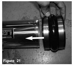
Attach 4" hump hose to injen intake tube. Do not tighten.
