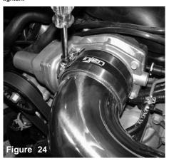
Tighten clamps on straight hose using 8mm nut driver.
