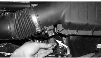
Depress the tab and pull the electrical harness connector from the mass air flow sensor.
