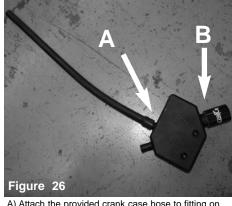
A) Attach the provided crank case hose to fitting on catch can that has the hole cut out.
