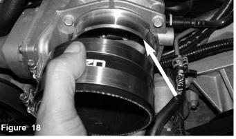
Attach 3.5" straight hose to throttle body with clamps provided and secure. Tighten only on throttle body using 8mm nut driver.
