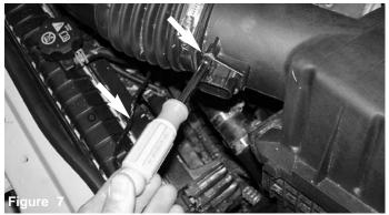
Loosen and remove the two screws holding the mass air flow sensor in the sensor housing
