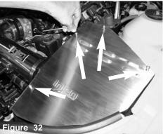
Secure cover using M6 button head screws and tighten using 4mm allen key.
