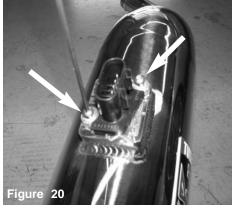
Secure MAF sensor using M4 button head screws. Tighten using 2.5mm allen key.
