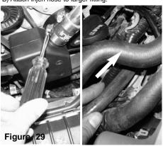
A) Tighten all clamps on catch can. B) Attach crank case line to engine.
