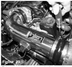
Tighten clamps on hump hose using 8mm nut driver.
