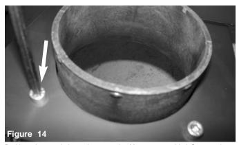
Position adaptor to holes and secure using M6 screws provided. Secure using 6mm allen key.
