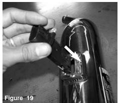
Install MAF sensor into new injen intake tube.
