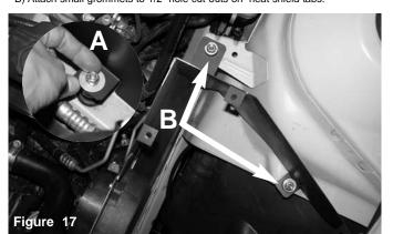
A) Secure housing tab to stand-off mount using washer and M6 nut. B) Secure the 2 upper tabs using factory M6 nuts. Secure housing using 10mm socket and ratchet.
