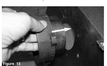
Install filter adaptor to inside of heat shield.
