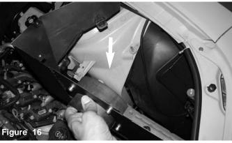
Install and position heat shield into vehicle.
