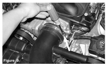
Loosen the throttle body clamp over the air intake duct.
