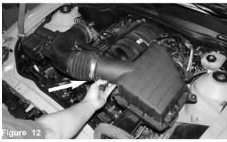
The air box cleaner is now ready to be moved from the engine compartment. Remove crank case line.
