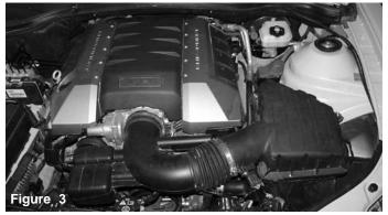
Stock air intake cleaner and air ducts shown in this picture. Before getting started with the installation, disconnect the negative battery terminal.
