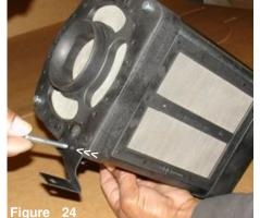
The m6 x 65mm bolt is loosened and removed from
