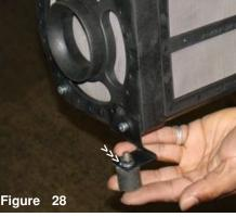
Use the m8 flange nut to secure the vibra-mount to the bracket as shown above.
