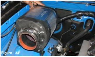
Now that the power box has been installed, press the 4 inch straight hose over the velocity stack end. Once the 4 inch hose is in place, place two power bands (.462) over the hose and tighten the clamp on the velocity stack end.
