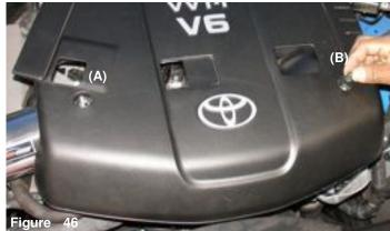
When the engine cover has been cut and fitted, lower the cover over the intake 1/4-20 aluminum stud(A) and intake plenum stud (B). Use one stack nut and 1/4-20 nut provided to secure the cover to the intake stud and the intake plenum stud.
