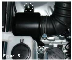
Loosen and remove the two m8 bolts that secures the resonator box to the fender well.
