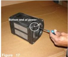
Position the power box with the rectangular screen facing forward and the air inducer facing towards you. Loosen the m6 x 45mm bolt as shown above.
