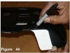
Place the pattern on the edge of the engine cover and use a marker to trace a line around the pattern.
