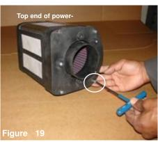
Turn the power box so that the velocity stack is now facing you. Loosen and remove the m6 x 65mm bolt that secures the body.
