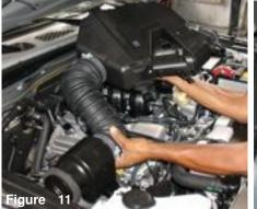
The entire air box cleaner and resonator box is now removed from the engine compartment. The entire air cleaning unit will not be used for this installation. Page 2 of Part# PF2057
