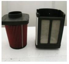
The velocity stack with filter is now out of the power box body.
