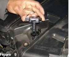
The mass air flow sensor is now lifted from the air box cleaner. The mass air flow sensor will be installed on the intake further on in the instructions.
