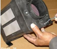
The m6 x 65mm bolt is screwed and fastened to the velocity stack base.
