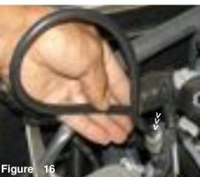
Press the 18 inch, 4mm vacuum line over the fuel pressure regulator port.
