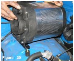
The rear vibra-mount is inserted into the grommet hole, now set the velocity stack bracket over the vibra-mount after the rear vibra-mount has been set in the hole.
