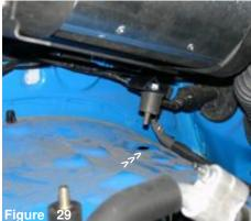
Lower the power box into the engine compartment, the rear vibra-mount fastened to the bracket is now inserted into the grommet hole location.
