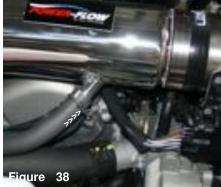
Once the breather hose has been properly installed over the 5/8 intake port, use the wire tension clamp to secure the breather hose in place.
