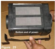
The saddle is placed under the power box ready to be attached.
