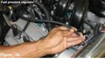
Press the 18  $\,$  -4mm vacuum line installed earlier on the fuel pressure regulator over the 3/16  $\,$  intake port.
