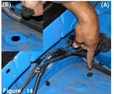
Remove the small rubber plug by the firewall (A). Pull the rubber plug out (B) This is where the bracket vibra-mount will be located, further in the instructions.
