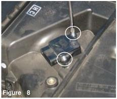
Unscrew the two bolts from the mass air flow sensor as shown above, then slowly pull the mass air flow sensor from the air box cleaner.
