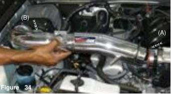
Insert the three inch end of the intake into the throttle body hose (A). Once the 3 side has been positioned in the throttle body hose, continue to insert the 4 end into the power box 4 inch straight hose (B).
