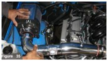
Now continue to insert the 4 inch intake end into the power box 4 inch straight hose as shown above (A) . Note the 1/4-20 stud placed over the intake (B) the stud must be facing up because this is where the engine cover will be attached.
