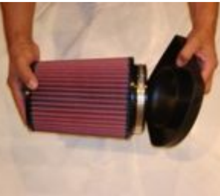
Once you have loosened the filter neck clamp, continue to pull the filter from the velocity stack.
