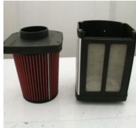
The velocity stack with filter is now out of the power box body.
