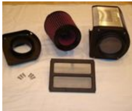
Here is a group shot of the components that goes into the power box. The filter and screen can now be cleaned with a simple shop-vac.
