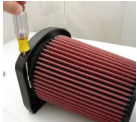
Loosen the clamp on the filter next in order to separate the filter from the velocity stack.
