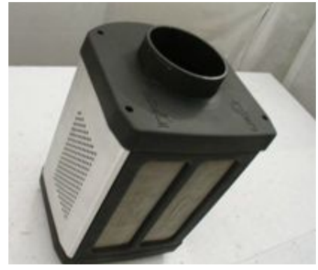
The four m6 x 20mm bolts have been removed from the top of the velocity stack.
