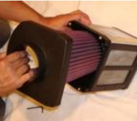
Here are the four-m6 x 20mm bolts that will be removed from the velocity stack base located on the corners of the base.
