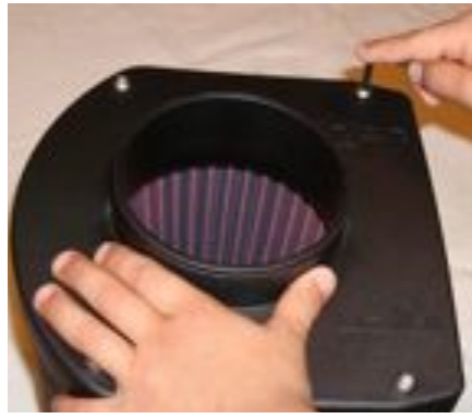
Unbolt the four-m6 x 20mm screws from the velocity stack base located to the center of the base. Now separate the base from the body.
