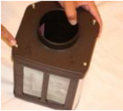
Here are the four-m6 x 20mm bolts that will be removed from the velocity stack base located on the corners of the base.
