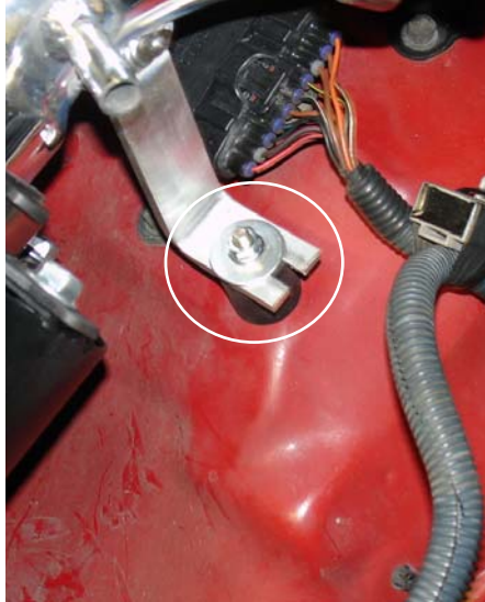
Once the secondary intake has been pressed into the 2 1/2" straight hose the intake bracket is secured using the m6 flange nut and fender washer.
