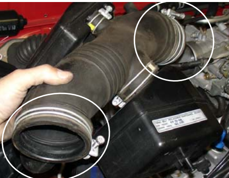
Loosen the two clamp located on each side of the air intake duct. Once the clamps have been loosened removed the entire air intake duct from the throttle body and air intake box.
