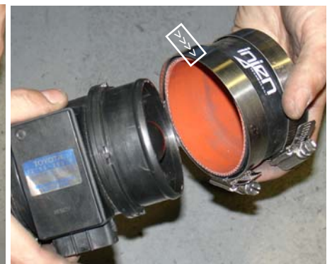
Press the 3" straight hose over the outlet end of the mass air flow sensor. Use two Power-clamps and tighten the clamp on the mass air sensor side.
