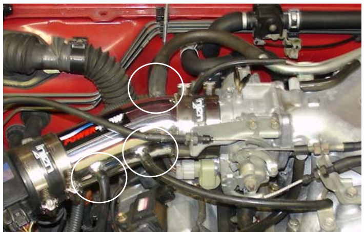
The vacuum lines that connect the pressure regulator port , power steering switch and the crankcase ports have all been installed.
