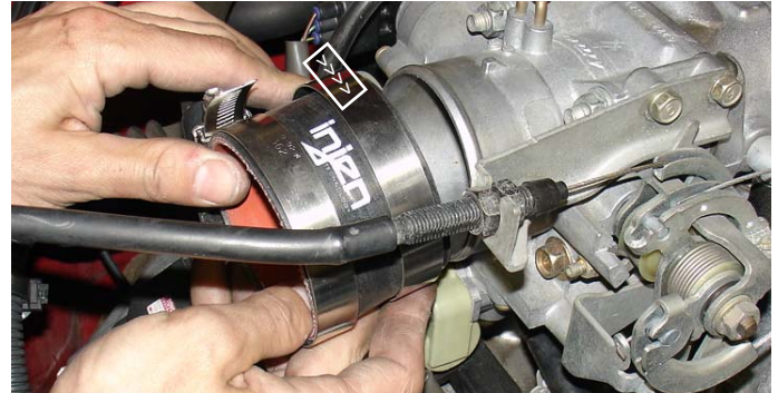
Press the 2 3/4" straight hose over the throttle body and use two power clamps on the straight hose, tighten the clamp located over the throttle body.
