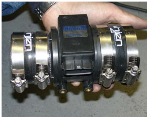
The mass air flow sensor is now assembled and ready for installation.
