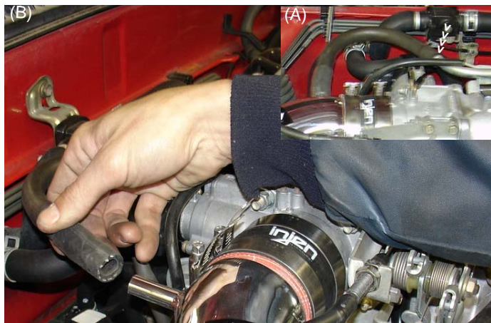
The stock crack case breather line is replaced with the 13" -10mm vacuum hose (A). Press one end over the crankcase breather port and connect the other end over the 1/2" intake port located by the firewall (B).
