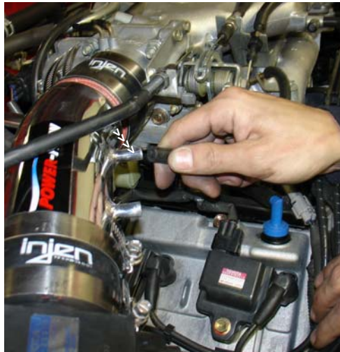
The hose just pressed over the fuel regulator port is connected to the first 3/8" port located on the primary intake.
