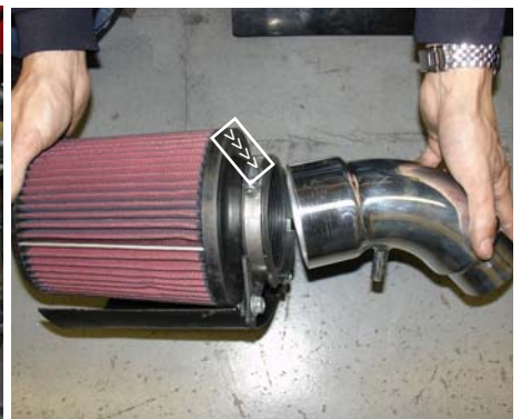
Press the 3 1/2" filter neck over the secondary intake as shown above. Once the intake has butted up against the filter neck continue to tighten the clamp. The Power-heat shield shown on the filter is an accessory not included in this kit.
