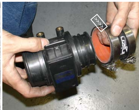
Press the 2 1/2" straight hose over the inlet side of the mass air flow sensor. Use two Power-clamps and tighten the clamp on the mass air flow sensor end.
