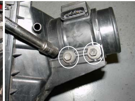
In order to remove the air mass sensor, the two m6 bolt will have to be removed.
