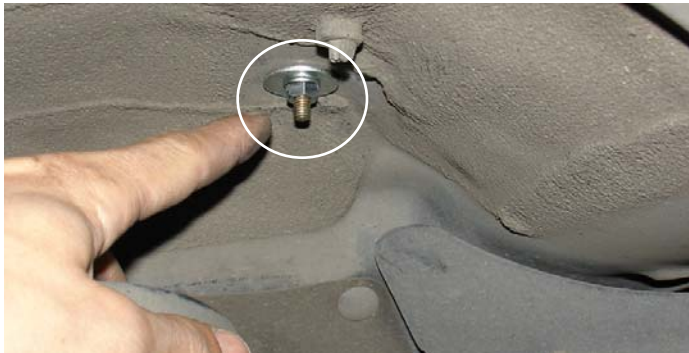
A shot of the m6 flange nut and washer from the wheel well securing the vibra-mount in place.
