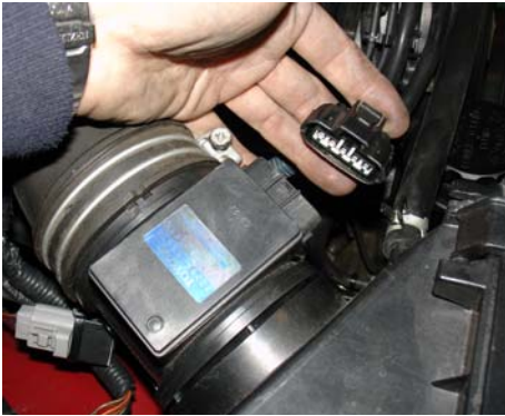
Disconnect sensor harness from the mass air flow sensor as shown above.
