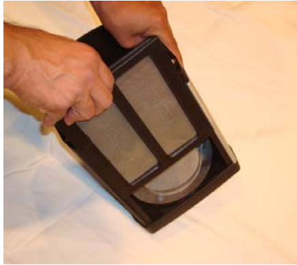
The rectangular pre-filter screen is now slipped out of the channel along the body of the power box.
