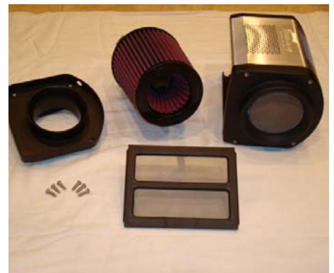
Here is a group shot of the components that goes into the power box. The filter and screen can now be cleaned with a simple shop-vac.
