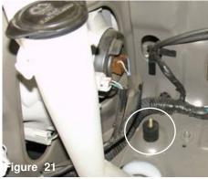
The first vibra-mount is now installed as shown above.
