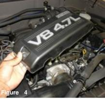
Once the flange nuts have been removed, continue to remove the cover from the engine compartment as shown above.
