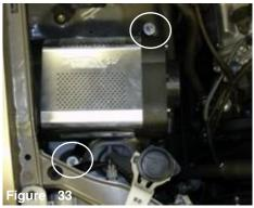
The Power box is now sitting flush over the vibramounts and a fender washer is placed over each vibra-mount.
