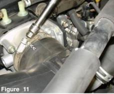
Loosen the hose clamp on the air duct connected to the throttle body.
