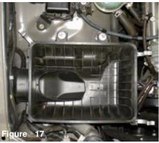
Remove the entire lower air box cleaner from the engine compartment.
