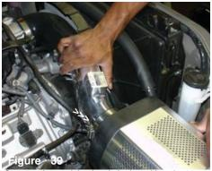
Once you inserted the throttle body end into the 90 degree elbow, insert the other end into the step hose located on the Power box.
