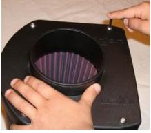
Unbolt the four- m6 x 20mm screws from the velocity stack base located to the center of the base Now separate the base from the main body.
