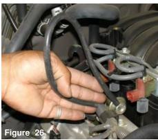
Press the new 16 - 4mm vacuum hose over the fuel pressure regulator port.
