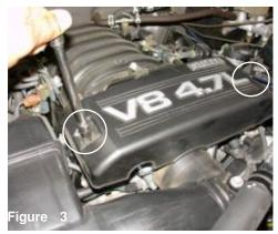
Loosen the two flange nuts on the engine cover in order to remove the cover.
