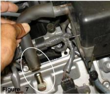
Unplug the crank case breather hose from the air crank case port as shown above.
