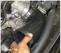
Place the power bands over each end of the silicone elbow. press the short end of the silicone elbow over the throttle body.
