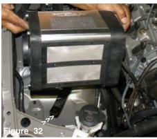
The assembled power box is lowered into the engine compartment. Align the mounting points on the bracket arms over the vibra-mounts.
