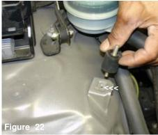
Screw the second vibra-mount is aligned over the wheel well bracket.
