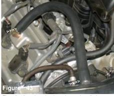
The 15 -15mm breather hose is now installed on both ends as shown above.
