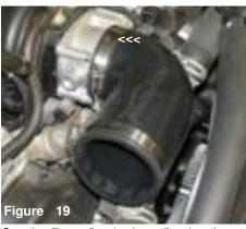
Once the silicone elbow has been aligned continue to semi-tighten power band over the throttle body end.
