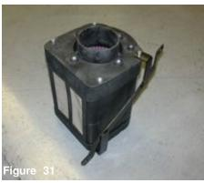
The mounting bracket is now installed under the power box.
