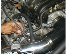
The fuel pressure vacuum line is pressed over the 3/16 intake port as shown above
