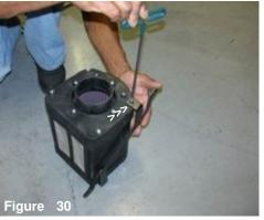
The 65mm bolt is tightened with an allen wrench.
