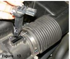
Carefully, remove the mass air flow sensor from the air sensor housing to be reused later in the instructions.
