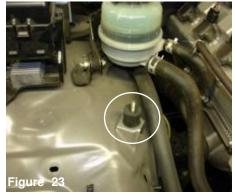
The second vibra-mount is now installed as shown above.
