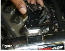
The mass air flow sensor is carefully lowered into the machined intake adapter.
