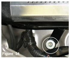
A n m6 flange nut is screwed over the front vibramount and fastened tight.
