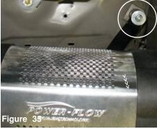
The last m6 flange nut is placed over the vibramount located behind the Power box.
