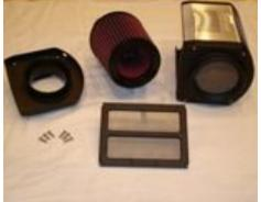
Here is a group shot of the components that goes into the power-box. The filter and screens can now be cleaned with a simple shop-vac.
