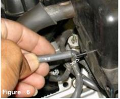
Disconnect the 4mm vacuum line located to the side of the air box cleaner.
