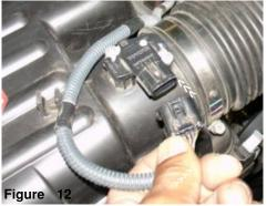
Unplug the electrical harness clip from the mass air flow sensor as shown above.
