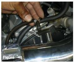
Press the stock 6mm hose over the center 3/8 intake port. Use the stock hose clamp to secure the line.
