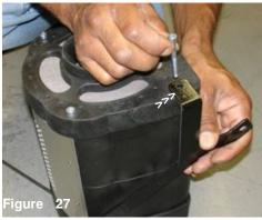
One 45mm bolt is removed from the top of the box. The bracket is place under the Power box and the 45mm bolt is aligned and screwed back in place as shown above.
