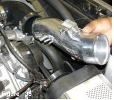
Insert the intake end with the vacuum ports into the 3 1/2 silicone as shown above.
