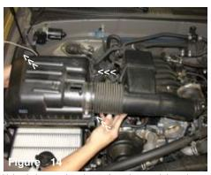
Unhook three spring clamps from the top air box cleaner. Once the hooks have been removed, continue to detach the air box top from the lower air box cleaner.
