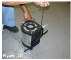
The 45mm bolt is tightened with an allen wrench.
