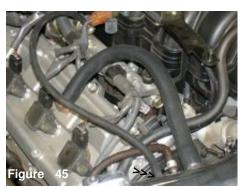
The 16 -4mm fuel pressure vacuum hose is now installed.
