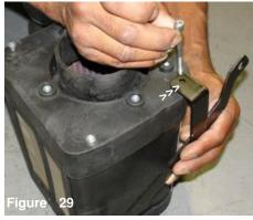
Remove the 65mm bolt from the velocity stack base. Align the bracket to the hole and insert the 65mm bolt back in place.
