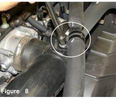
Unscrew the nut and bolt the hose clamp that secures the hose over the radiator.
