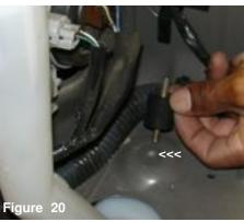
The first vibra-mount is aligned to the pre-tapped hole located behind the head lamp.
