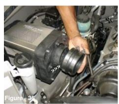
Place one .462 and a .412 power band over the silicone step hose. Press the 3 3/4 side over the velocity stack as shown above.
