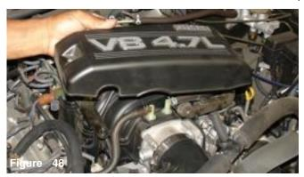
Align the engine cover to the intake bolt while lowering the cover over the intake. Use the 1/4-20 oval flange nut to fasten the cover to the intake threaded bolt. The engine cover will fit snug over the intake as shown above.
