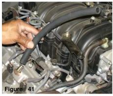
Press the 15 -15mm hose over the crank case breather port
