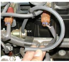
The stock 6mm hose is removed from the fuel pressure regulator.
