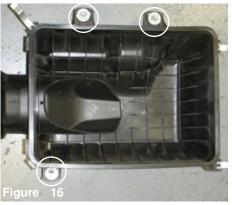
Once the air filter panel is removed, there are three bolts that will be removed in order to detach the lower air box cleaner.
