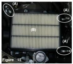
The three spring clamps shown above are unhooked from the top air box cleaner (A). Remove the air filter panel once the top has been removed (B).
