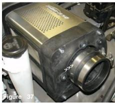
The step hose is now flush over the velocity stack base. Tighten the .462 power band on the velocity stack outlet.
