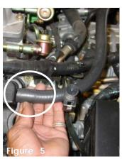
Press one end of the 16"-15mm breather hose over the port located on crankcase.
