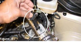
Remove the stock mass air flow sensor from the stock intake box and press it into the machined adapter located on the intake.
