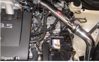
Top shot of the cold air intake installed.
