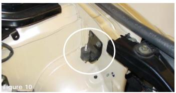
Installation of the vibra-mount: Screw the m6 vibra-mount into the brace located on the driver side fender well. Screw the vibra-mount in until it bottoms out.
