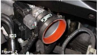
Press the 3 1/8" straight hose over the throttle body and use two clamps, tighten the clamp on the throttle body at this point (A).
