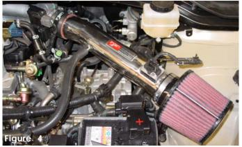
In order to prevent hydro-locking on rainy days, we strongly recommend you place the filter on the primary end of the intake. The cold air intake can be converted into a shortram whenever necessary for a little peace of mind.
