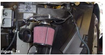
Press the filter over the end of the secondary intake and tighten the clamp located on the filter neck.
