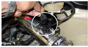
Press the harness clip over the mass air flow sensor until you hear it snap in place.
