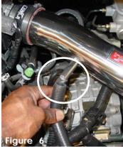
Press the remaining end on the breather over the long port on the intake.
