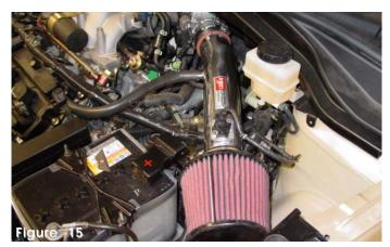
Here is another view of the cold air intake being converted into a shortram.
