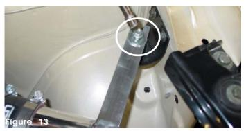
Line up the bracket on the intake to the vibra-mount stud. Use the m6 flange nut and fender washer to hold the entire intake in place.
