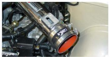
Installation of the secondary intake: Press the remaining 3" straight hose over the end of the primary intake and use two clamps, tighten the clamp on the intake side.
