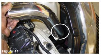
Take the secondary intake and insert it into the resonator opening. Begin to align the secondary intake to the primary intake.
