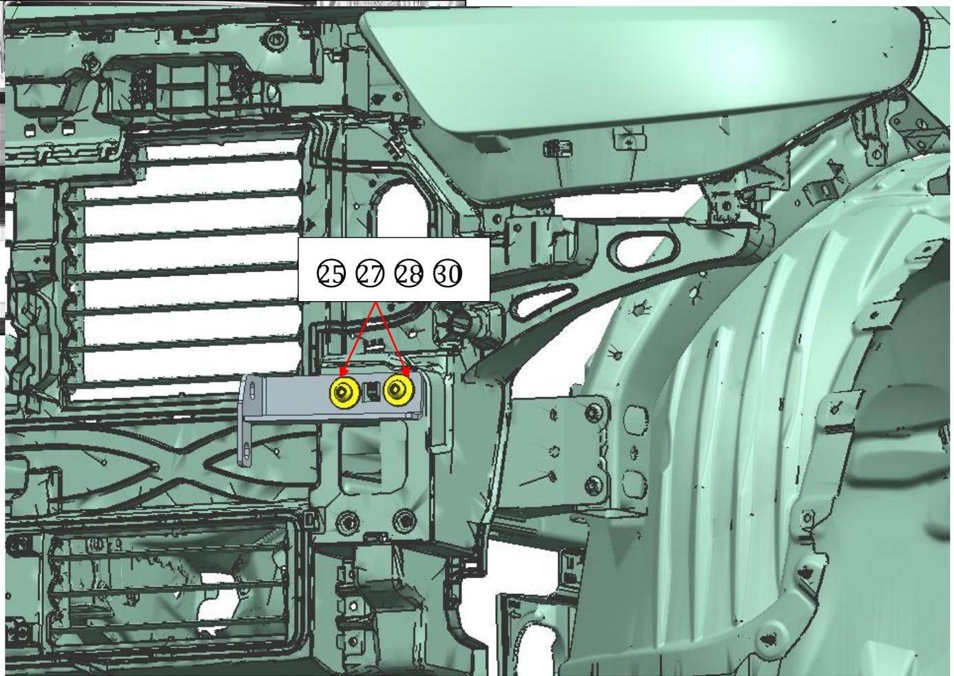
Then connect Bottom Support Brackets to Upper Brackets with standard parts ①⑨ ②① ②② ②④.
