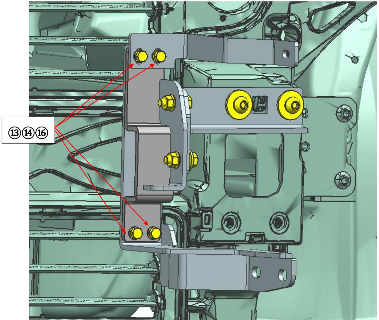
**Step3:** Reinstall the plastic front bumper. Need to cut off the place where the Lower Brackets against the intake grille.
