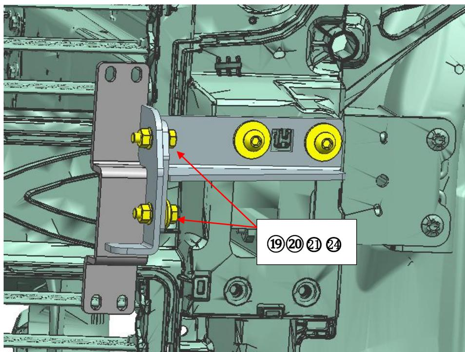
Finally, use standard parts to fix Top Support Brackets and Lower Brackets on the four mounting positions of the Upper Brackets.
