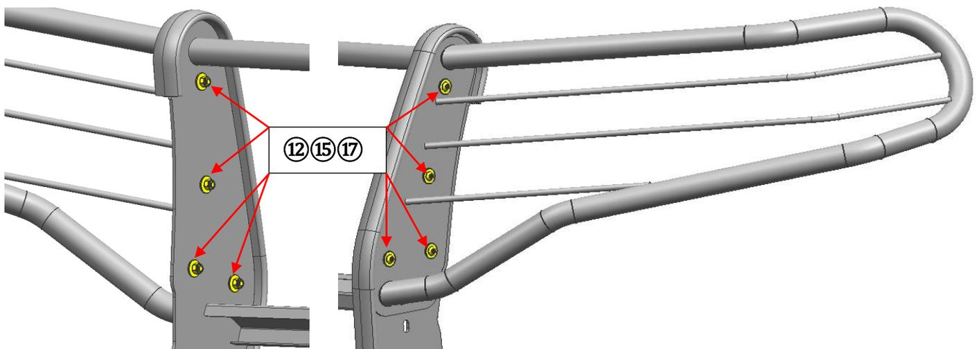
**Step 2:** Remove the original plastic front bumper. Fix the Bottom Support Brackets with standard parts ②⑤ ②⑦ ②⑧ ③①. (P.S.: The following installation steps show only the left side, but the installation method is consistent from left to right)
