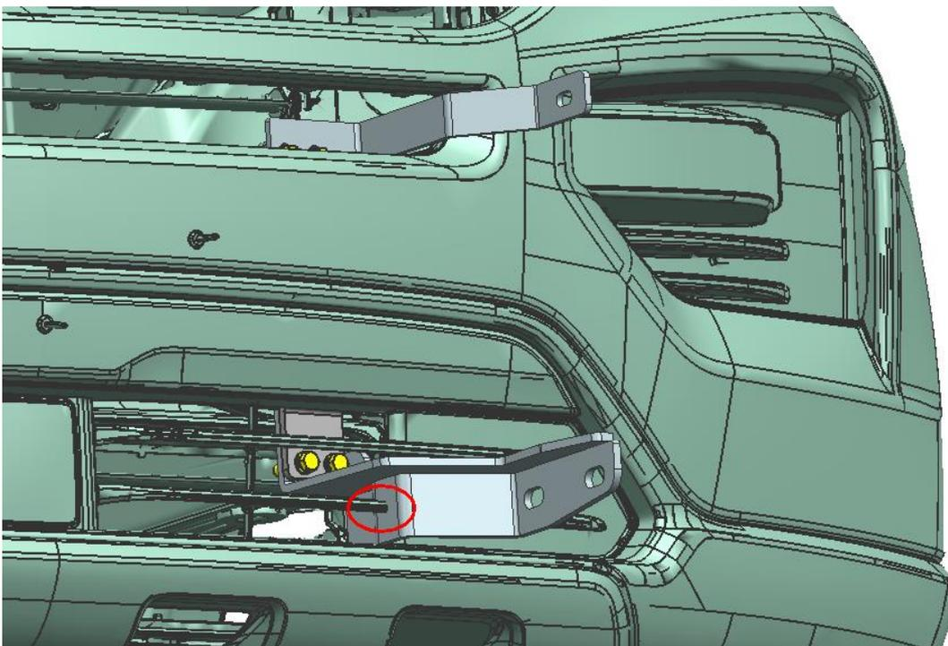
**Step4:** Finally, install the whole grille guard to the Top Support Brackets and Lower Brackets as shown in the figure. Adjust it to an appropriate position, and then tighten the standard parts.
