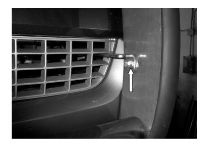
**STEP 8.** ALIGN THE GRILLE GUARD ASSEMBLY WITH THE FRONT OF THE VEHICLE AND TIGHTEN ALL MOUNTING NUTS AND BOLTS.
