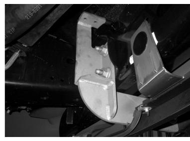
**STEP 4.** INSERT 1122AD UPPER BRACKET THROUGH THE OPENING IN THE GRILLE, AND ATTACH IT TO 1122BD LOWER BRACKET USING THE 5/16" HEX HEAD BOLTS. (FINGER TIGHTEN ONLY).
