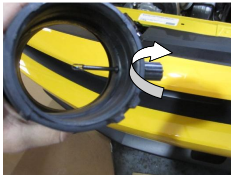
Remove the factory ATS by twisting and pulling up and out.
