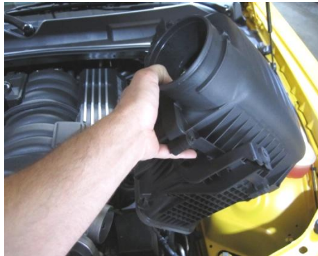
Remove the factory air box and duct.
