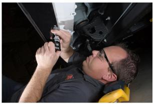
**STEP-6:** Apply a sealant (silicone adhesive) to the previously drilled pilot hole. This helps to seal the drilled hole.
