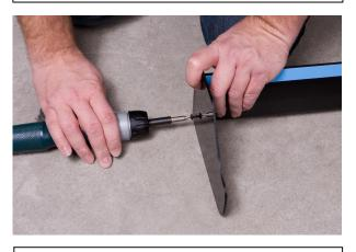
STEP-2: Assemble splash guards to the tab on cab and rear flares using the #6 screws. (Smaller screws) DO NOT OVERTIGHTEN!! (IMPORTANT NOTE: The hardware kit provided contains #6 and #10 screws. ONLY #6 screws should be used to attach the splashguards to the RockerFlare.)
