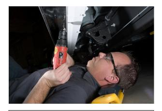
STEP-7: Using a drill, with a Phillips head bit, run #10 screws into the 1/8" pilot holes previously drilled. Do not over tighten. (NOTE: If the RockerFlares do not come with predrilled expansion holes, mount the flare and drill 1/8 inch holes spaced about 12 to 16 inches apart thru plastic and metal. Then follow with ½ inch holes just through the plastic to allow expansion and contraction. (This is very important).
