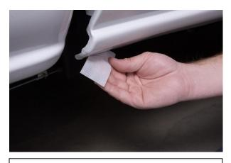
STEP-1: Clean the rocker panel mounting area with alcohol wipes provided. The rocker panel condition and preparation is very important to get a good bond to the flares. The rocker panel area where the flare will mount should be free from dirt, rust, grease, and wax. Temperature must be at least 60 degrees.
